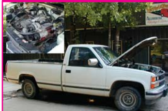
1989 Chevrolet / 1500 Series This is one of S&P's shop trucks using the 1993 LT1 Motor with 4L60 Transmission.
