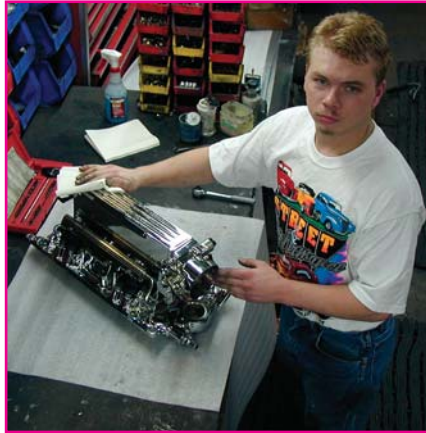
Final assembly of the new "RamJet Injection"
