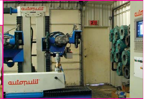
One of three automatic CNC robotic polishing machines
