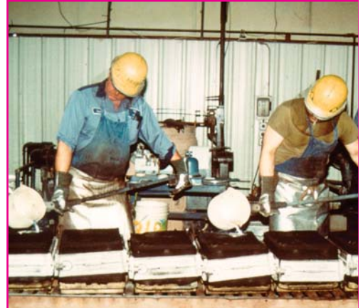
Pouring of 713 aluminum alloy in the foundry
