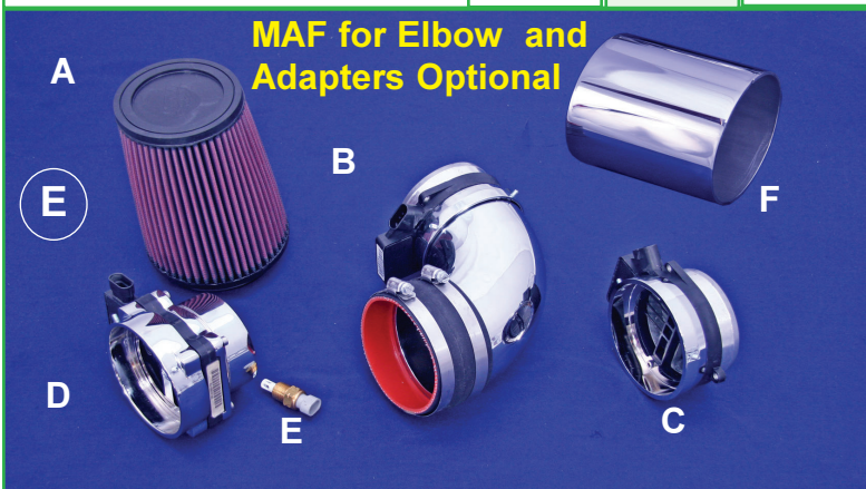
LS2 Air Cleaner using 5 Pin MAF adapter with PCV Vent
