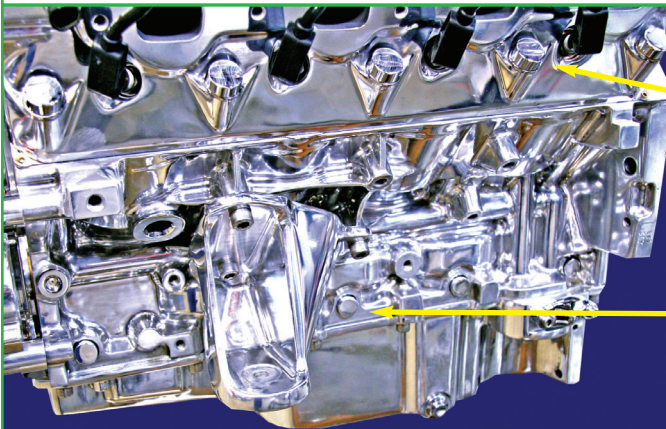
Tight Upper Passenger Side Alternator and Low Passenger Side Air (Must use IROC Balancer)
