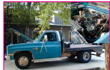
1981 Chevy 1-Ton "Hauler" Larry Sanders, Chrome Shop Foreman of S&P, dropped in the 454 BBC Motor including the S&P BB Multi-Port Fuel Injection Unit.
