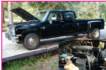
1986 Chevrolet / Dually "For Towing" S&P's shop trucks using the 454 BBC Motor with S&P BB Multi-Port Fuel Injection Unit.
