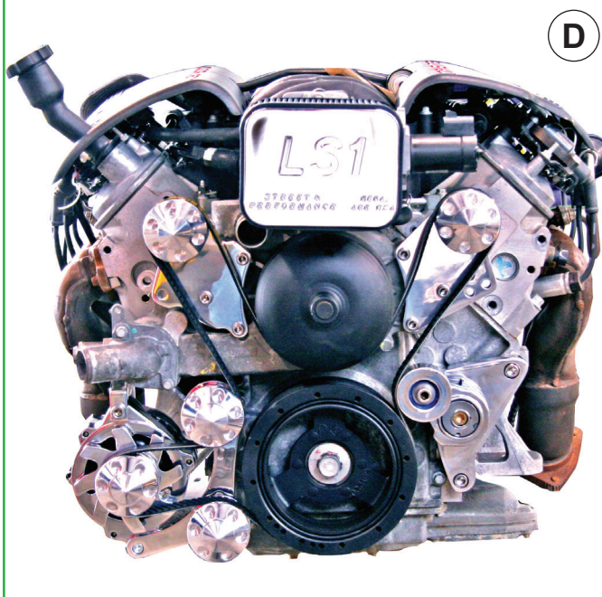
Tight Upper Passenger Side Alternator (Must use IROC Balancer)
